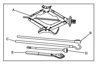
The tools you will be using include the jack (A), jack handle extension (B), jack handle (C), wheel wrench (D), and the ratchet (E).
